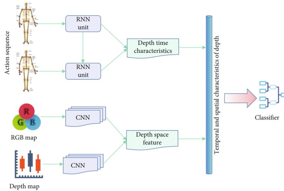
Figure 1.3 Architecture Diagram of Deep Space-time Feature Motion Recognition [20]
