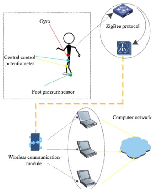
*Figure 1.2 Schematic Diagram of the Wearable Sensor Network [18]*
