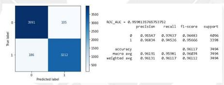
Figure 4.0.10: confusion matrix and precision, recall, f1-score, and support scores for Stacking ensemble learning method.
