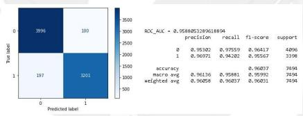
Figure 4.0.7: the confusion matrix and precision, recall, f1-score, and support scores for the Boosting ensemble learning method.
